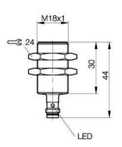
Inductive Sensors BES 516-367-G-E5-Y-S 49 M18x1 x 44 normally-closed Sn=8mm shielded
